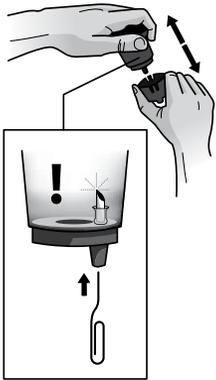
**2. Cleaning the Funnel**—The Funnel can be removed from the K-Cup® Pack Holder by pulling on it until it pops off (fig. 9). The Funnel is dishwasher safe. To replace it, just snap it back onto the K-Cup® Pack Holder Assembly.
