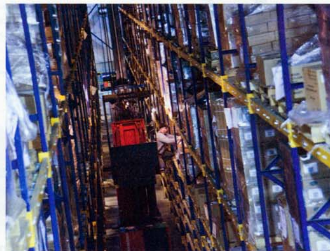
▲ Green Mountain Coffee's warehouse features pick tunnels that have lights that flash when a product needs to be picked.
