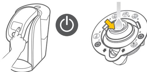
2. Lift Handle, properly place Brewer Maintenance Accessory in Pod Holder with printed arrows pointing down.
