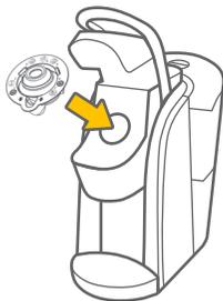
3. Raise and lower the Handle five times to loosen and remove any coffee grounds retained in your brewer's Entrance Needle.
