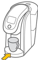
2. Lift and lower the Handle. Do not place a Keurig® brand pod in the Pod Holder.
