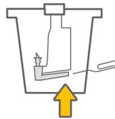
3. After all the pieces are cleaned, place the Base then the Pod Holder assembly into the Brew Head. lower the Handle.
