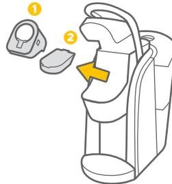
3. Press the release buttons on both sides of the Pod Holder Assembly.
