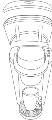
The water reservoir lid and water reservoir should be periodically cleaned with a damp, soapy, non-abrasive cloth and rinsed thoroughly. The water reservoir lid and water reservoir should not be put into the dishwasher. Do not dry the inside of the water reservoir with a cloth as lint may remain.
